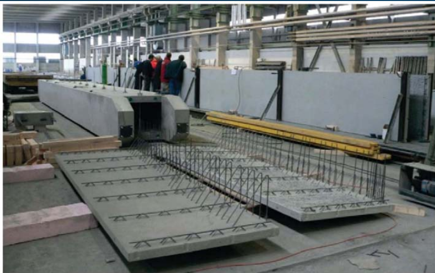
Production of prefabricated elements at the Austrian precasting company Oberndorfer
