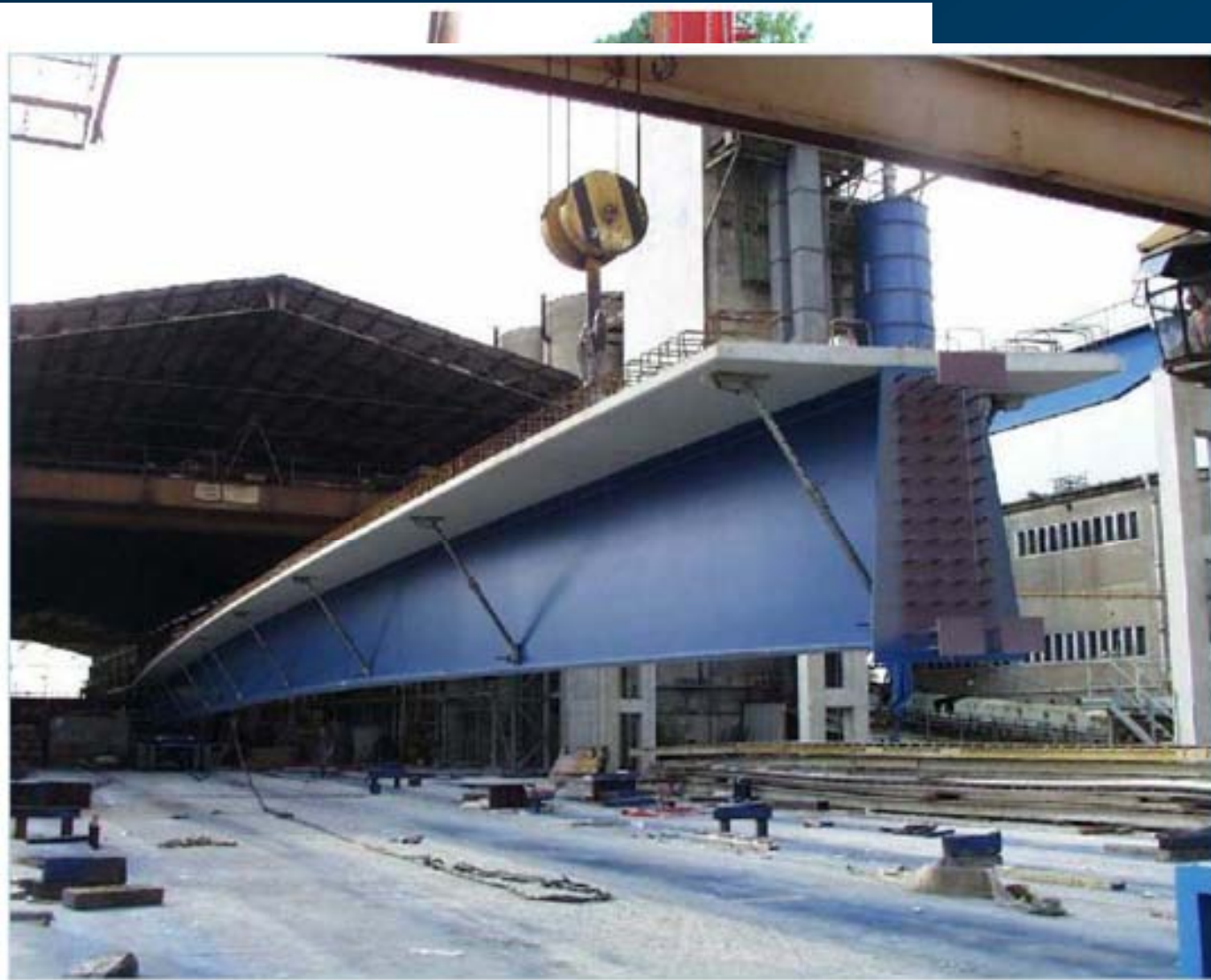
“Ready to transportation” VFT girder in the factory.
