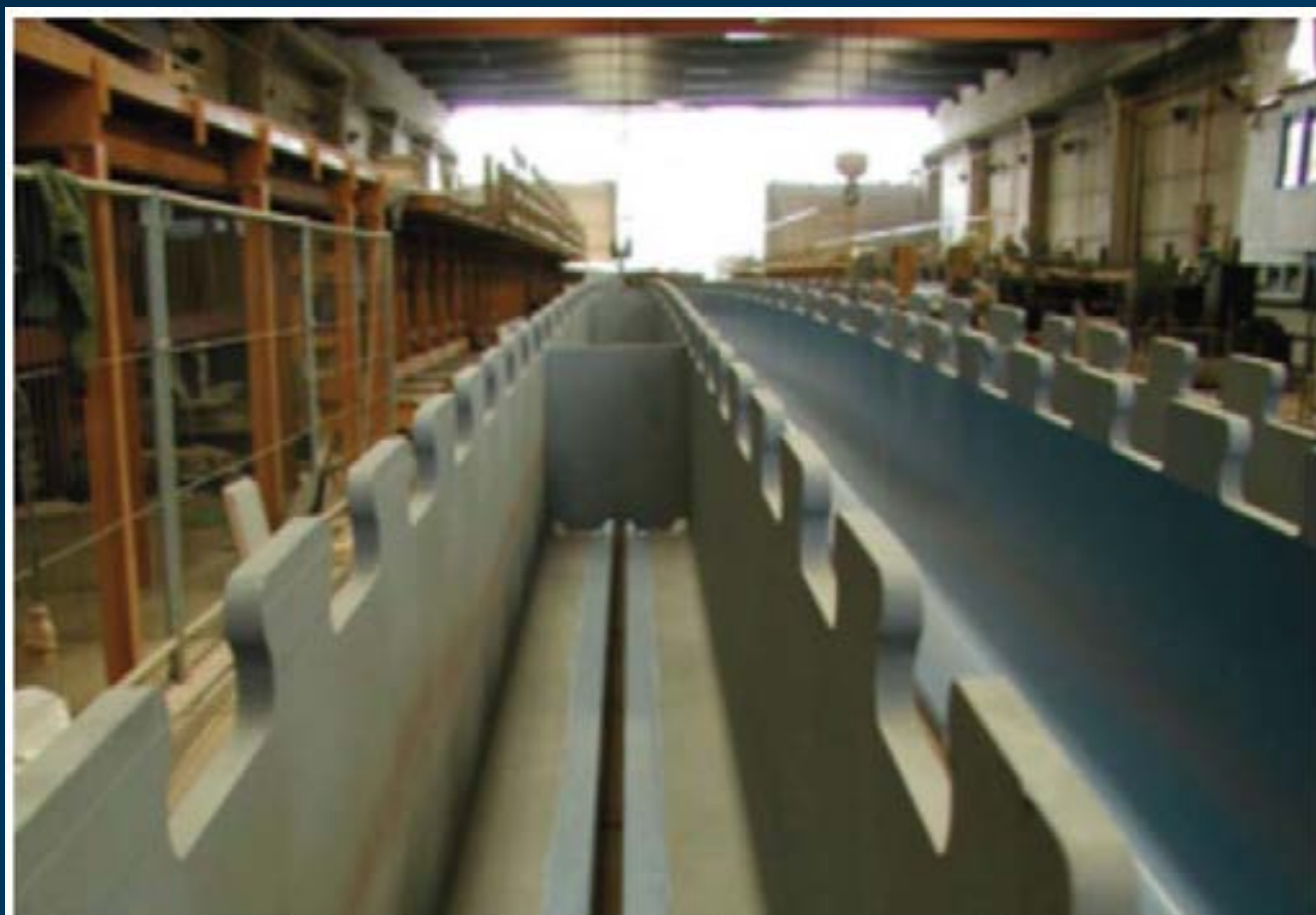
Cut (halved) rolled sections with PZ-geometry of the dowels and coating in the prefabrication plant
